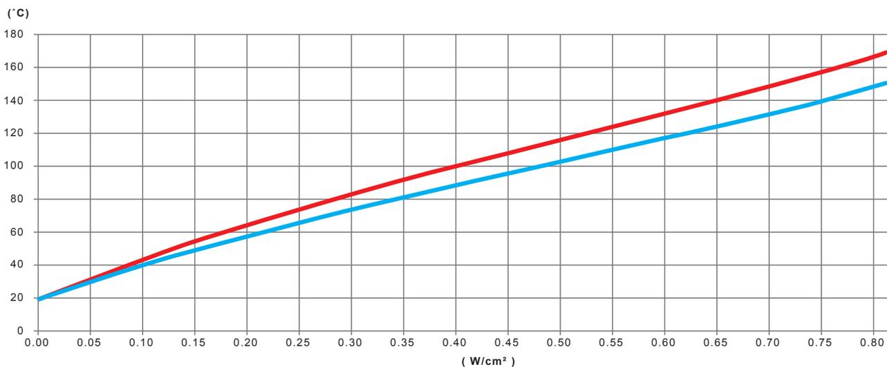
Variation, in function of the power in  $W/cm^2$  of the silicone heating tape, of the temperature of the wall of a **stainless steel tube, not thermally insulated**
