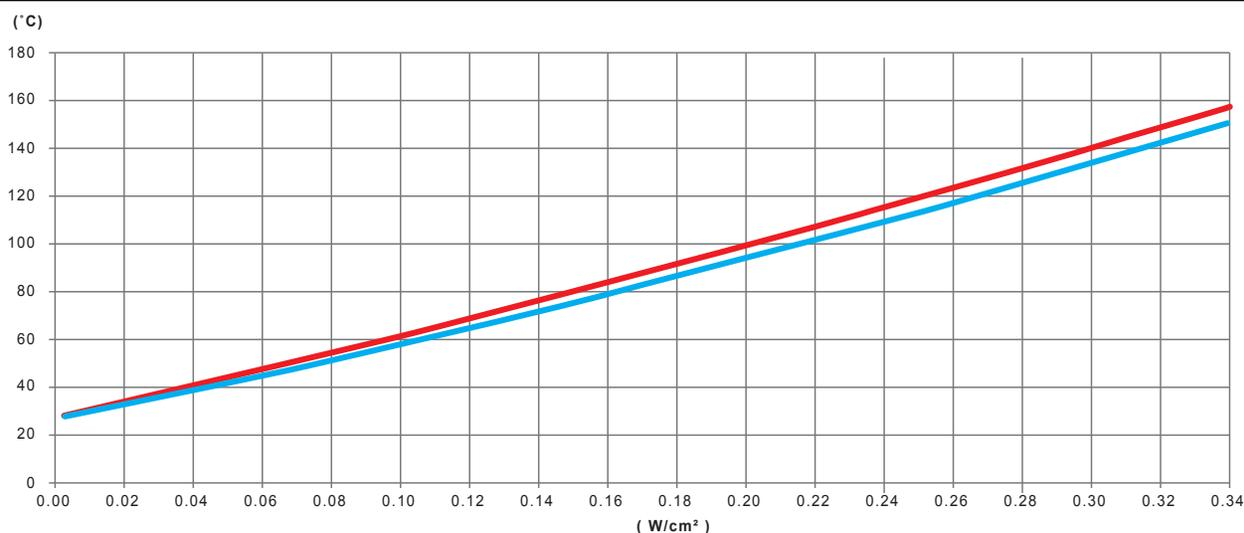
Variation, in function of the power in  $W/cm^2$  of the silicone heating tape, of the temperature of the wall of a **stainless steel tube, thermally insulated with 20mm of PVC-NBR foam**
