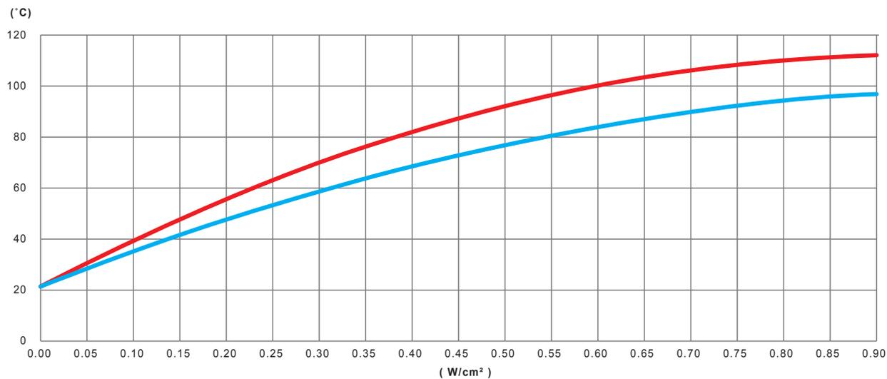
Variation, in function of the power in  $W/cm^2$  of the silicone heating tape, of the temperature of the wall of a **stainless steel tube, filled with non-circulating water and not thermally insulated**
